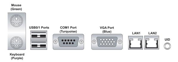
Figure 5-2. Rear Panel I/O Ports
